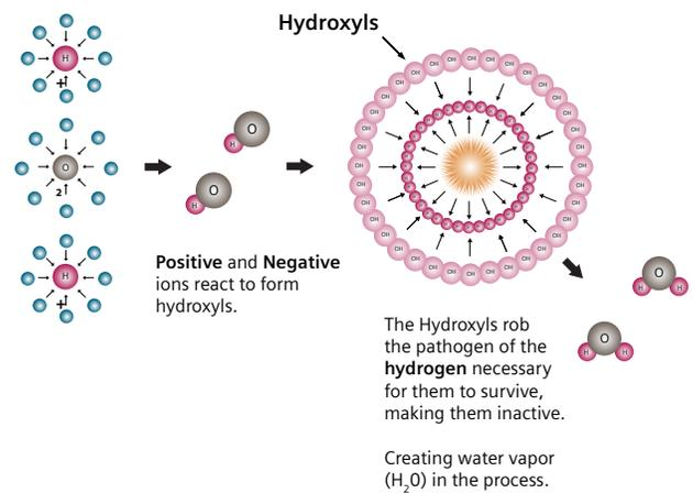
Ozone-Free Needlepoint Bipolar Ionization artificially creates millions of positive and negative ions and releases them into the forced air circulation of an HVAC system travelling into spaces inside building(s).
